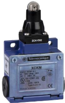
**Limit switch, Limit switches XC Standard, XCKM, steel roller plunger, 1NC+1 NO, slow break, Pg11**
